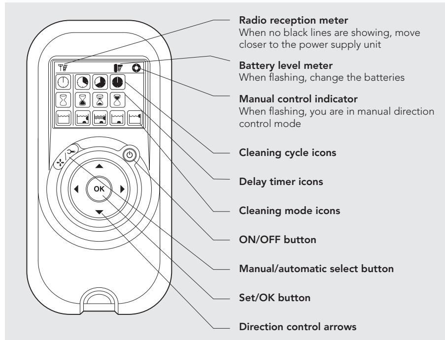
The remote control unit (RCU) offers two operation modes – Automatic mode and manual direction control mode.
