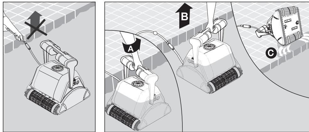
Using the floating cable, bring the Pool Cleaner to the pool's edge.
